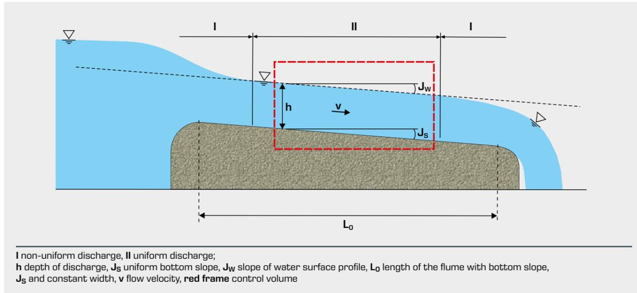
In uniform open-channel flow the discharge depth  $h$  remains equal, i.e. parallel to the bottom. This also means that the flow velocity  $v$  remains constant.
