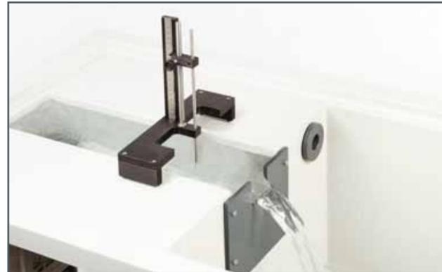
Sharp-crested overfall at a measuring weir
