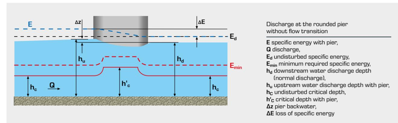
Discharge at the rounded pier without flow transition
