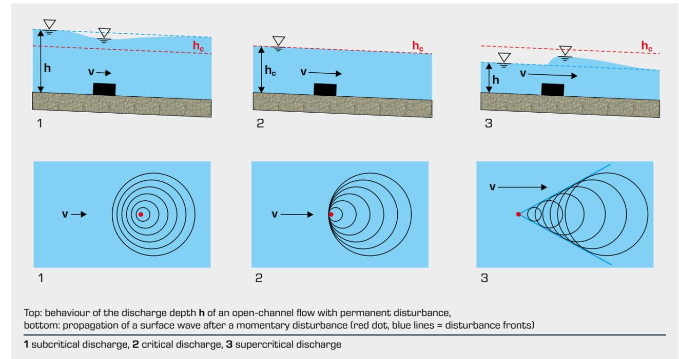
Top: behaviour of the discharge depth  $h$  of an open-channel flow with permanent disturbance, bottom: propagation of a surface wave after a momentary disturbance (red dot, blue lines = disturbance fronts)
