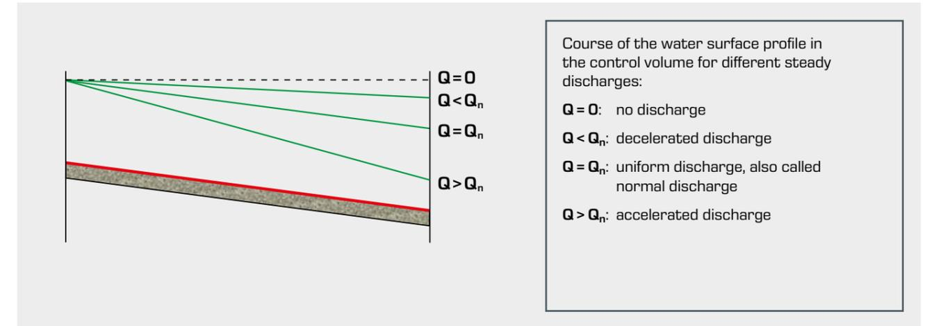
When considering energy head on the control volume we can resort to **Bernoulli's equation** and the **continuity equation**.
