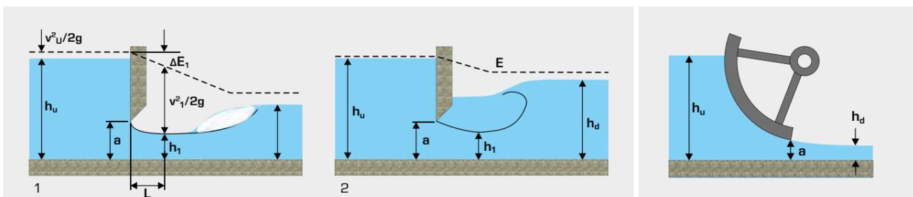
Discharge under a sluice gate
