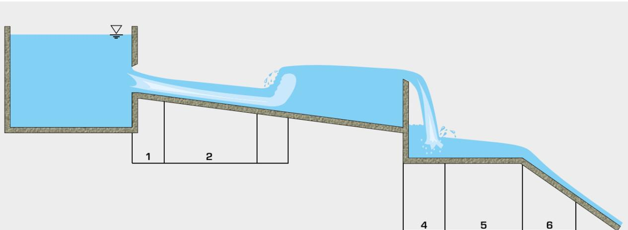
1 rapidly varied discharge under a gate, 2 gradually varied discharge, 3 hydraulic jump (rapidly varied), 4 weir overfall (rapidly varied), 5 gradually varied discharge, 6 non-uniform flow at a change of slope
