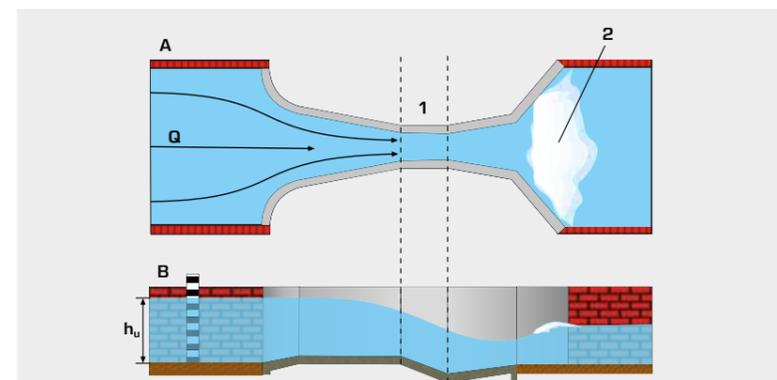
A plan view of venturi or Parshall flume, B side view of a Parshall flume;
