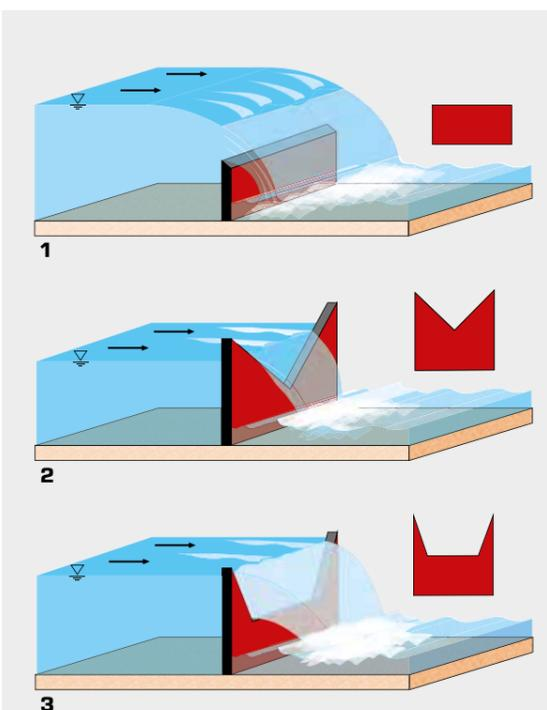
Flow over typical measuring weirs in side and plan view
