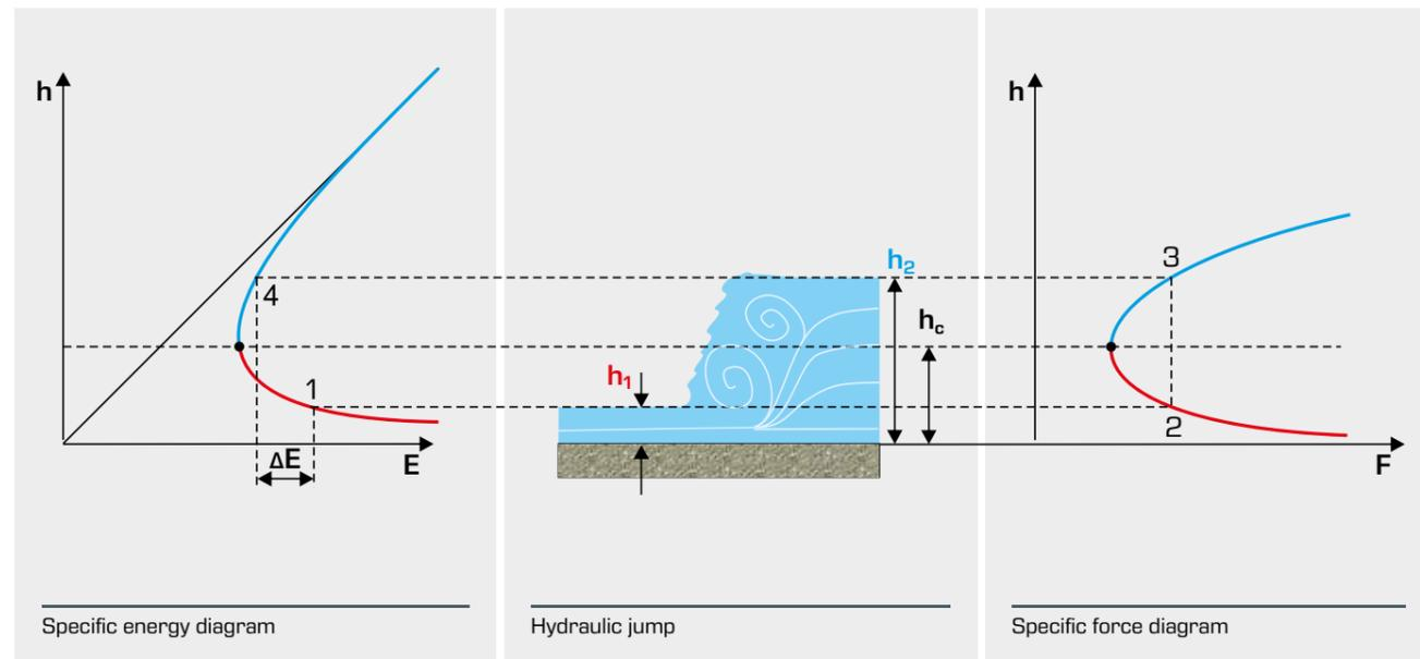
The discharge depth  $h_1$  is entered in the specific energy diagram and the specific force diagram (points 1 and 2). To determine the discharge depth  $h_2$  after the hydraulic jump, the sequent depth to  $h_1$  is determined graphically in the specific force diagram (point 3). The specific forces  $F_1$  in point 2 and  $F_2$  in point 3 are
