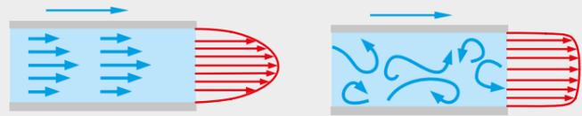
Velocity profile in fully developed flow
