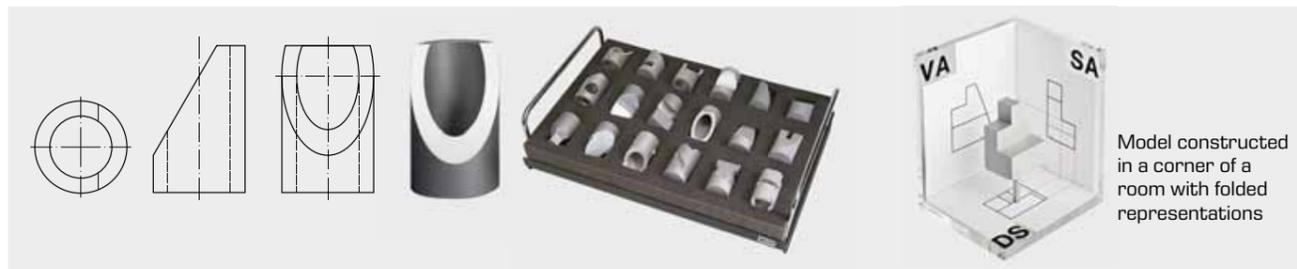
Model constructed in a corner of a room with folded representations
