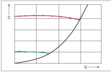
Pump characteristics: H head, Q flow rate; red: characteristics at n=2900min<sup>-1</sup>, green: characteristics at n=1450min<sup>-1</sup>, black: system characteristic
