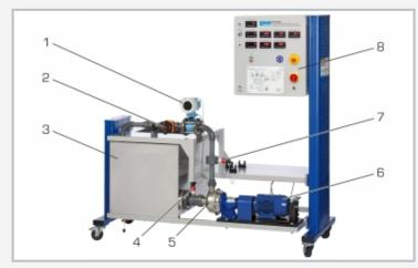
1 electromagnetic flow meter, 2 flow control valve, 3 storage tank, 4 ressure sensor at pump inlet, 5 centrifugal pump, 6 drive motor including measurement of torque, 7 pressure sensor at pump outlet, 8 switch cabinet with displays and controls
