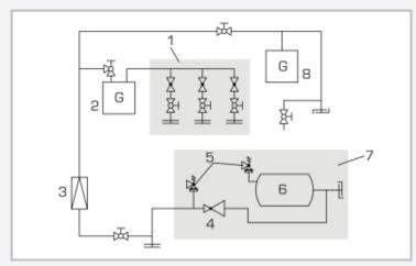
Process schematic: 1 leak simulation, 2 gas meter, 3 gas pressure controller, 4 air pressure controller, 5 safety valve, 6 pressure tank, 7 compressed air supply, 8 gas meter
