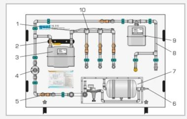
1 pipe section leak simulation, 2 ball valve, 3 gas meter with 2 connections, 4 gas pressure controller, 5 ball valve, 6 compressed air connection, 7 compressed air supply, 8 pipe section with gas socket and gas connection with ball valve, 9 gas meter with 1 connection, 10 valve
