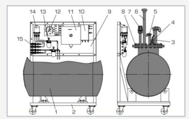
1 oil tank, 2 frame, 3 filler pipe with seal, 4 combination fitting, 5 dip stick tube with seal, 6 tank ventilation, 7 overfill protection, 8 dome cover, 9 fittings panel, 10 vacuum leak detector, 11 leak liquid tank, 12 level gauge with liquid leak detector, 13 oil filter, 14 automatic ventilation, 15 oil connections
