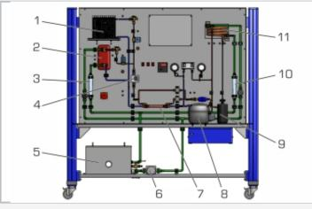
1 finned tube heat exchanger as evaporator, 2 plate heat exchanger as evaporator, 3 heating water flow meter, 4 refrigerant flow meter, 5 water tank, 6 water pump, 7 tubular heat exchanger as superheater, 8 compressor, 9 receiver, 10 cooling water flow meter, 11 coaxial coil heat exchanger as condenser
